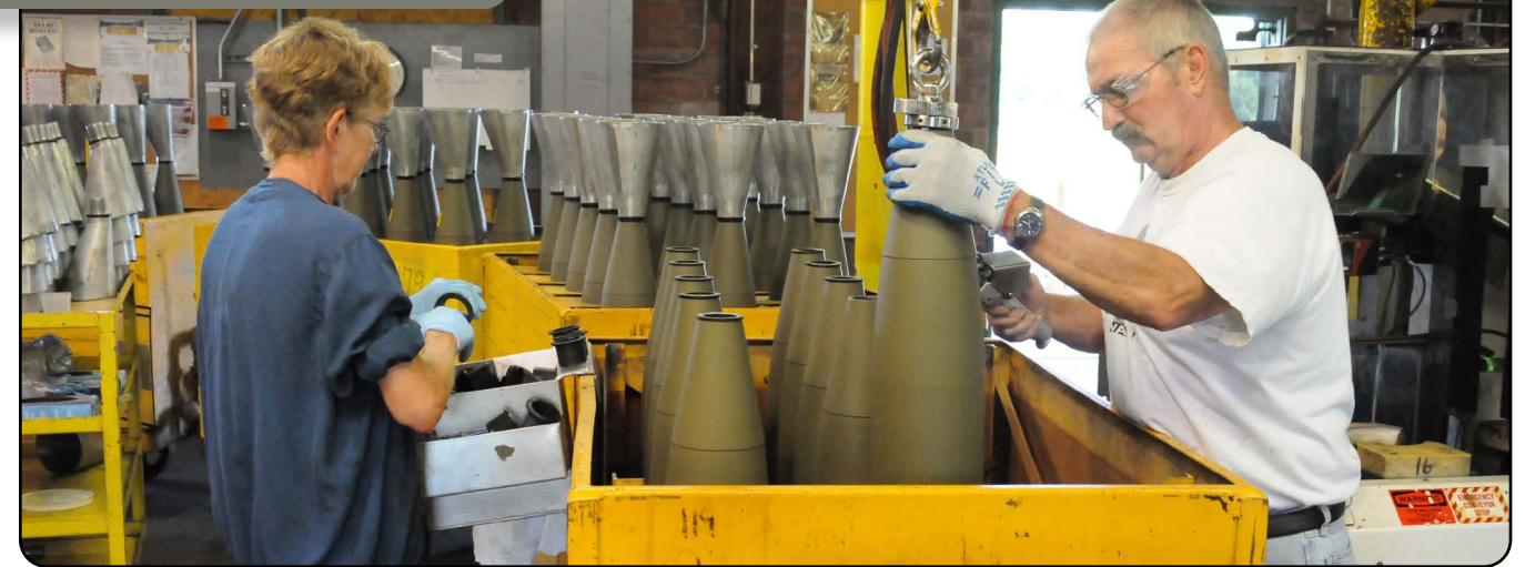
Contractor employees at IAAAP prepare 155 mm artillery rounds to be filled as a part of the load, assemble and pack operation. (U.S. Army photo by JMC)
