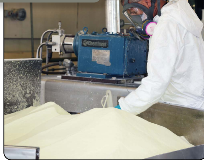
A contractor employee for Holston Army Ammunition Plant prepares explosives on a charging table to be bagged and placed into a drum. (U.S. Army photo by HSAAP)
