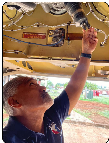
READINESS: U.S. Army Aviation and Missile Command Logistics Assistance Representative Galen Cajigal instructed four new maintainers on how to identify, inspect, and make necessary repairs on a CH-47F atf transmission filter. (U.S. Army photo by Katie Nelson)
