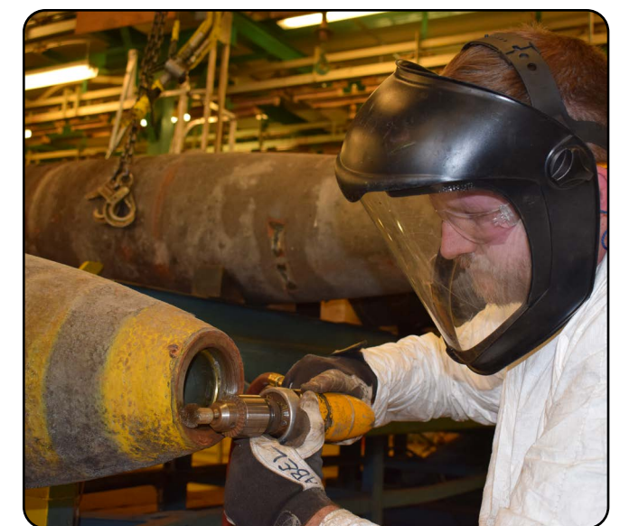
BOTTOM: Crane Army Ammunition Activity renovates MK84 bombs by replacing degraded thermal coating. This saves valuable taxpayer dollars and ensures warfighters always have quality munitions. CAAA specializes in conventional munitions support for U.S. Army and joint force readiness, including storage, quality control, shipment preparation, distribution, production and demilitarization. (U.S. Army photo by CAAA)
