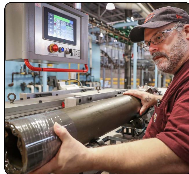
A consulting engineer is shown inspecting a CNC machined cartridge case. The machining step is critical to final interface of the case within the gun weapon system at QCCCF at the U.S. Army's Rock Island Arsenal, Rock Island, Illinois. (U.S. Navy photo by Matthew Poynor)
