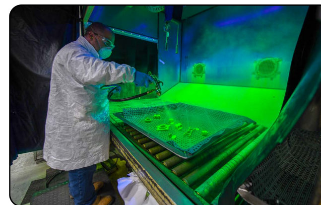
CCAD artisan Paul Zaklukiewicz, Non-Destructive Tester applies a concentrated fluorescent oil penetrant to the aircraft component to help detect defects under black light. (U.S. Army photo by Ervey Martinez)
