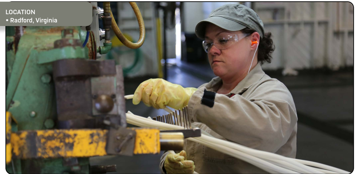
A RFAAP employee feeds solvent propellant into a cutting machine during production. (U.S. Army Photo by RFAAP)
