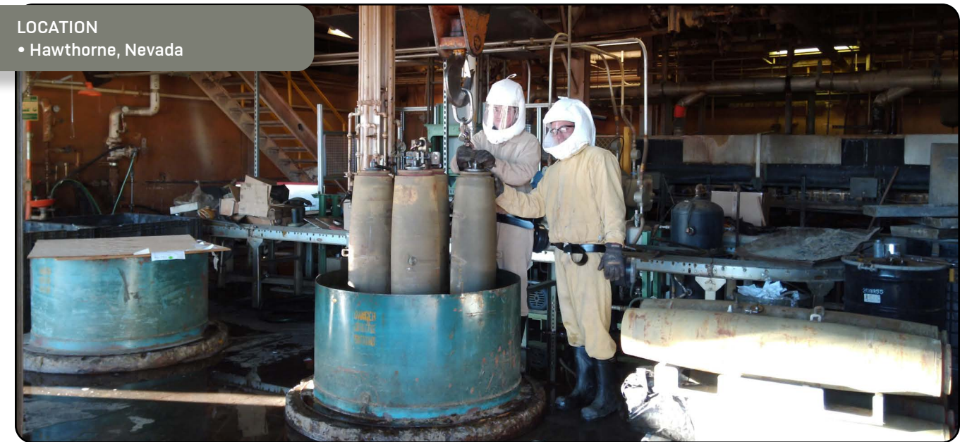
Contractor employees at Hawthorne Army Depot lower obsolete ammunition stockpile items into a belt flaker as a part of the decontamination and demilitarization process at HWAD. (U.S. Army photo by Sheila Viani)
